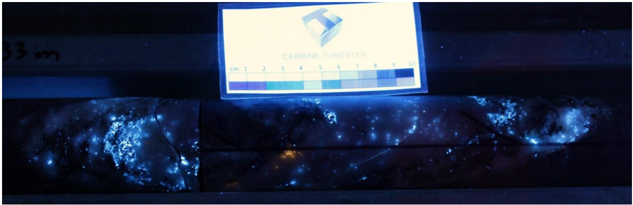
Photo 2: Hole MTCB005: 532.9-533.25 m. Strong scheelite mineralisation (Blue-White) and Powellite (Calcium Molybdenate – Golden Orange) fluorescing under short wave ultraviolet light.
