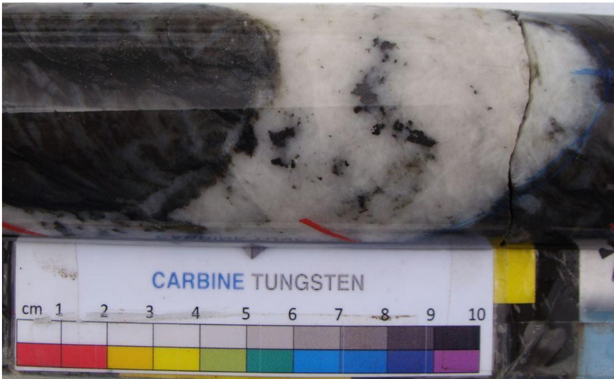
Photo 1: Hole MTCB005: 194 m. Narrow-bladed and disseminated Wolframite-bearing quartz vein with minor sulphide.
