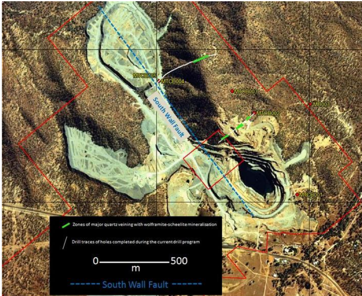
Figure 2. Plan view showing location of exploration drill holes MTCB 002, 004 and 005, and upward projects of intersection of sheeted quartz vein-hosted tungsten (wolframite and scheelite) mineralisation.
